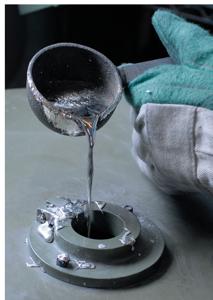
Apprentice Bryce Chandler pours molten pewter into a spoon mold. The machine spins it until the metal hardens.
