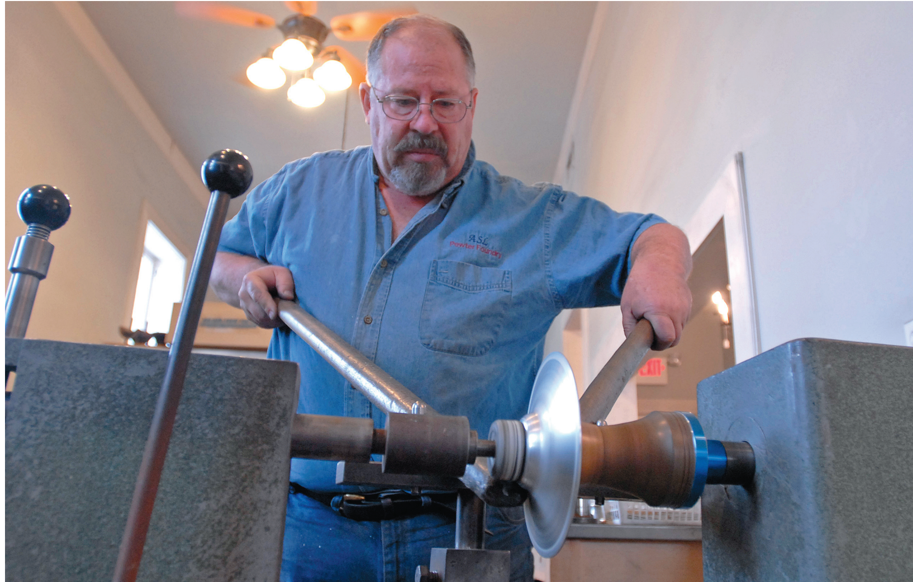
Above: On display in the shop are an inkwell set, tea set, punch bowl and other items crafted by the Hoopers. Left: Thomas Hooper uses a lathe in his workshop to create a bowl out of a flat, round piece of pewter. Below: Thomas trims a pewter bowl on another lathe.
